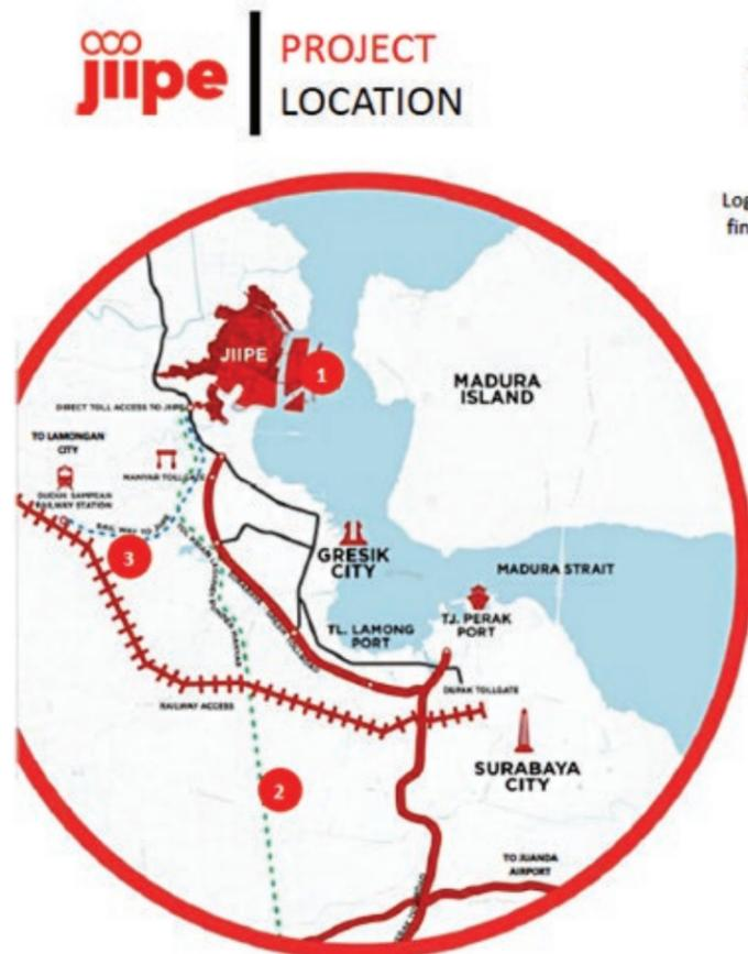
Located strategically in the mouth of Madura Straits, our attached port will be the deepest in East Java (-16 LWS). With 4 jetties and 6,200meter total berthing area, JIPE could cater large size bulk carriers until 100,000 DWT.
